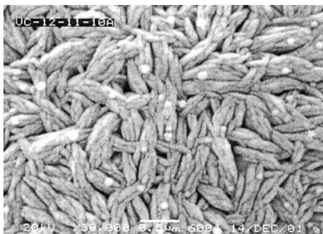
Fig. 2 SEM image of the larger granule in Fig.1 (30,000 times magnified)
